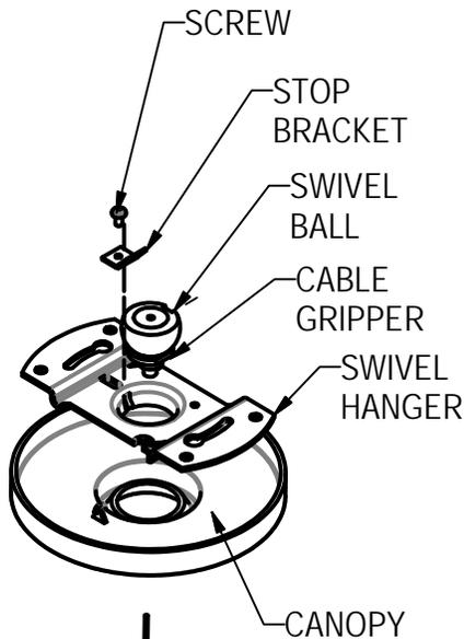
1. FEED AIRCRAFT CABLE UP THROUGH CANOPY, SWIVEL HANGER AND INSERT INTO CABLE GRIPPER.
